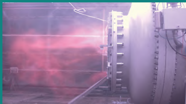
Fig. 3: Successful venting of a hydrogen explosion at REMBE Research+Technology Center GmbH.
