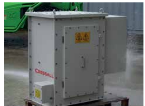
CRESSALL Cressall ATEX neutral earthing resistor (NER) undergoing an IP water test.
