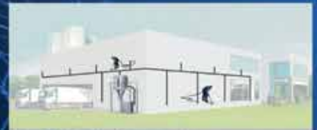
A schematic showing a typical Central Vacuum Cleaning System systems. They provide vacuum connection points for cleaning around the factory, plant or lab. Dust and debris is conveyed through the pipe system to a filter separator for safe disposal.
