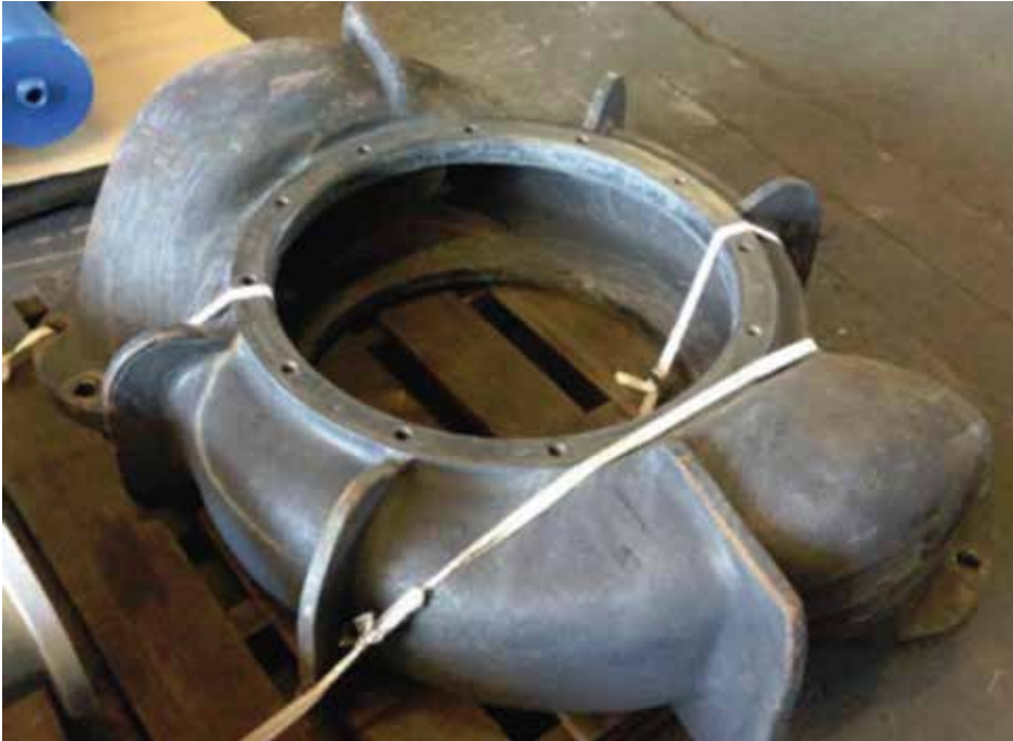
Above: Pump casing disassembled for repair
