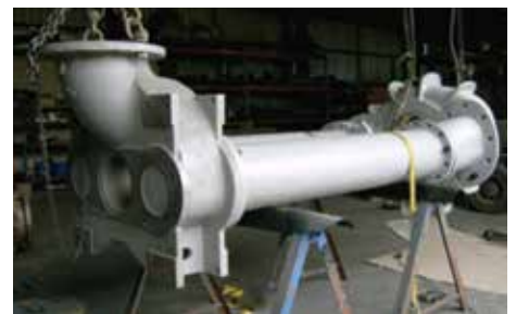
Above: External surface protected against high temperature
